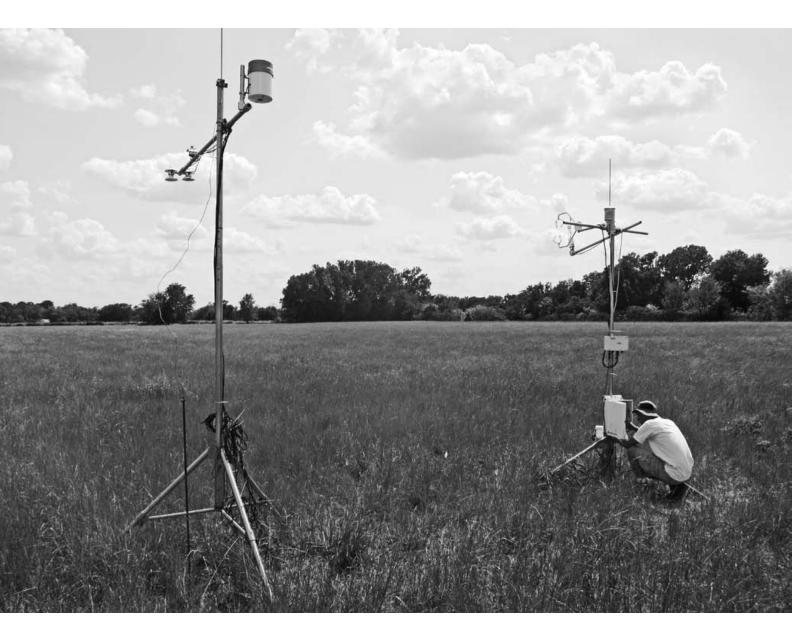
Eddy covariance equipment reads the flow of water vapor and carbon dioxide between the atmosphere and intermediate wheatgrass at The Land Institute. Lee DeHaan collects the data. Scott Bontz photo.
