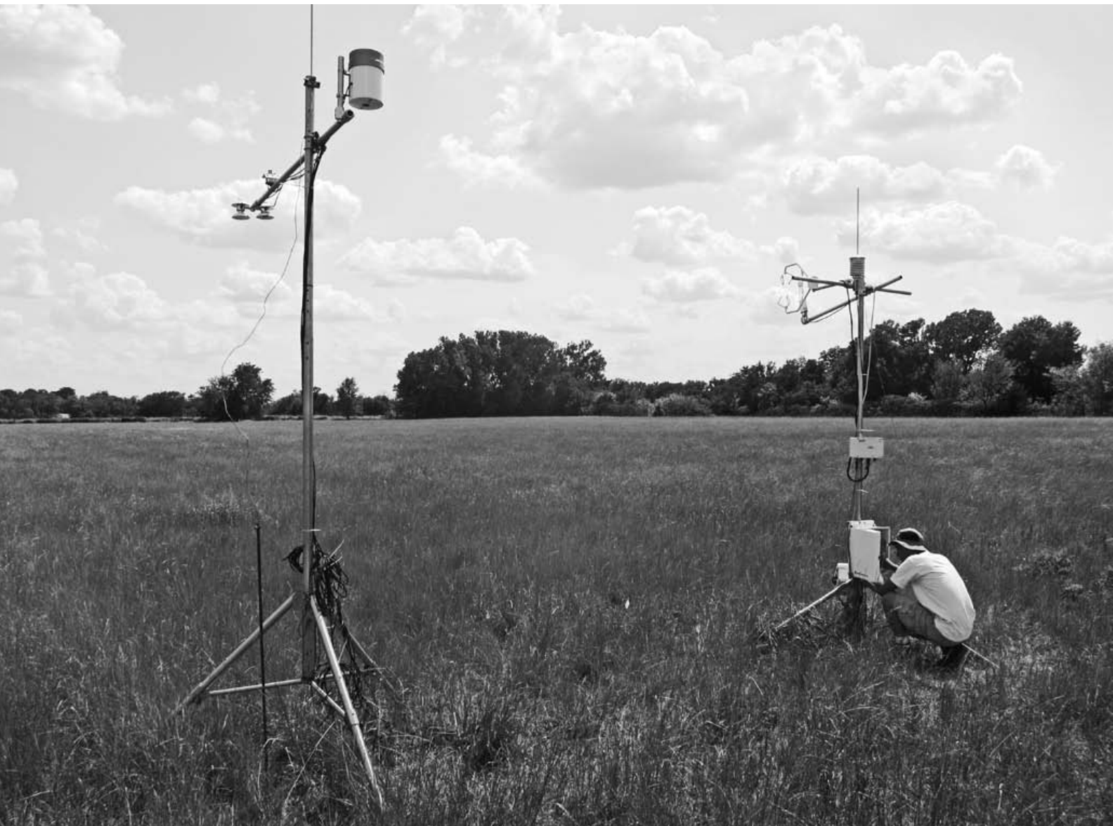
Eddy covariance equipment reads the flow of water vapor and carbon dioxide between the atmosphere and intermediate wheatgrass at The Land Institute. Lee DeHaan collects the data. Scott Bontz photo.
