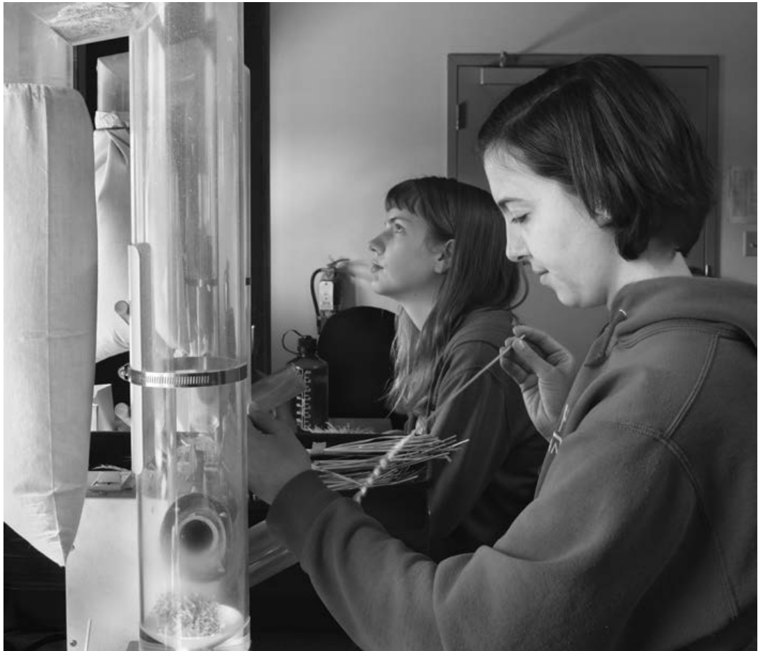
Jamie Ramsey, left, and Emma Hauser thresh the grain from individual heads and plants of perennial wheat. Air blows chaff up the clear tubes and into the bags at left. Seed is heavier and drops for collection. It then is measured to gauge the worth of the parent plant. For news on wheat progress, see the page 2 caption. Scott Bontz photo.
