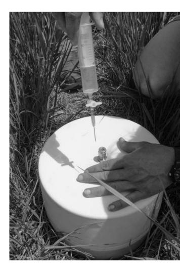
A cap traps nitrous oxide, a greenhouse gas, coming from soil where alfalfa and wheatgrass grow. The syringe is used to withdraw samples for analysis. This helps in study how soil changes while organisms and their relationships shift over the long haul of perennial plant growth. Scott Bontz photo.
