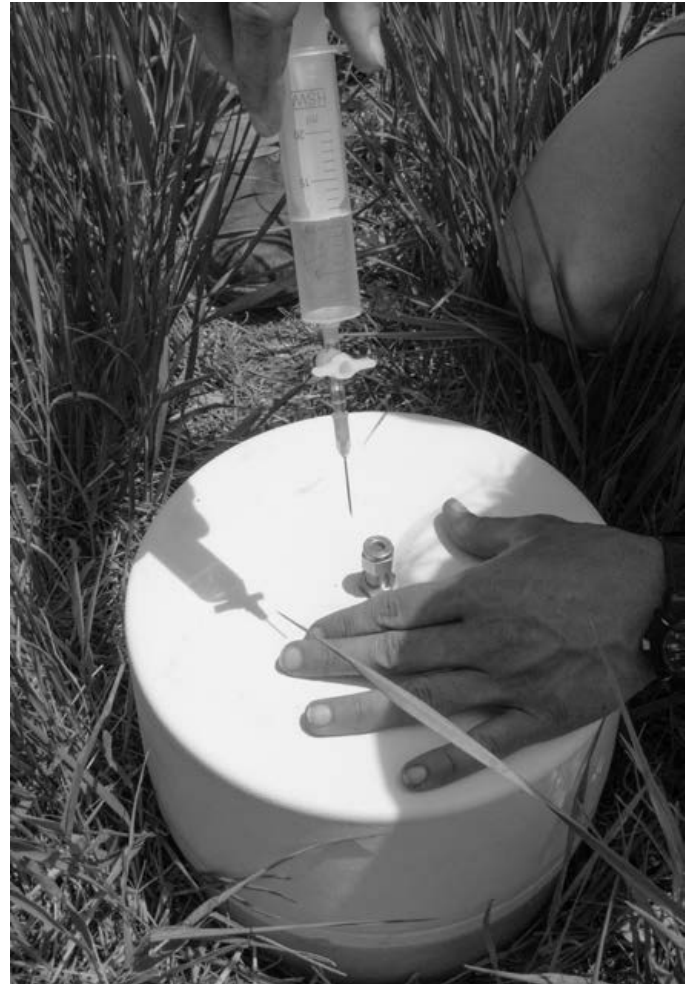
A cap traps nitrous oxide, a greenhouse gas, coming from soil where alfalfa and wheatgrass grow. The syringe is used to withdraw samples for analysis. This helps in study how soil changes while organisms and their relationships shift over the long haul of perennial plant growth. Scott Bontz photo.
