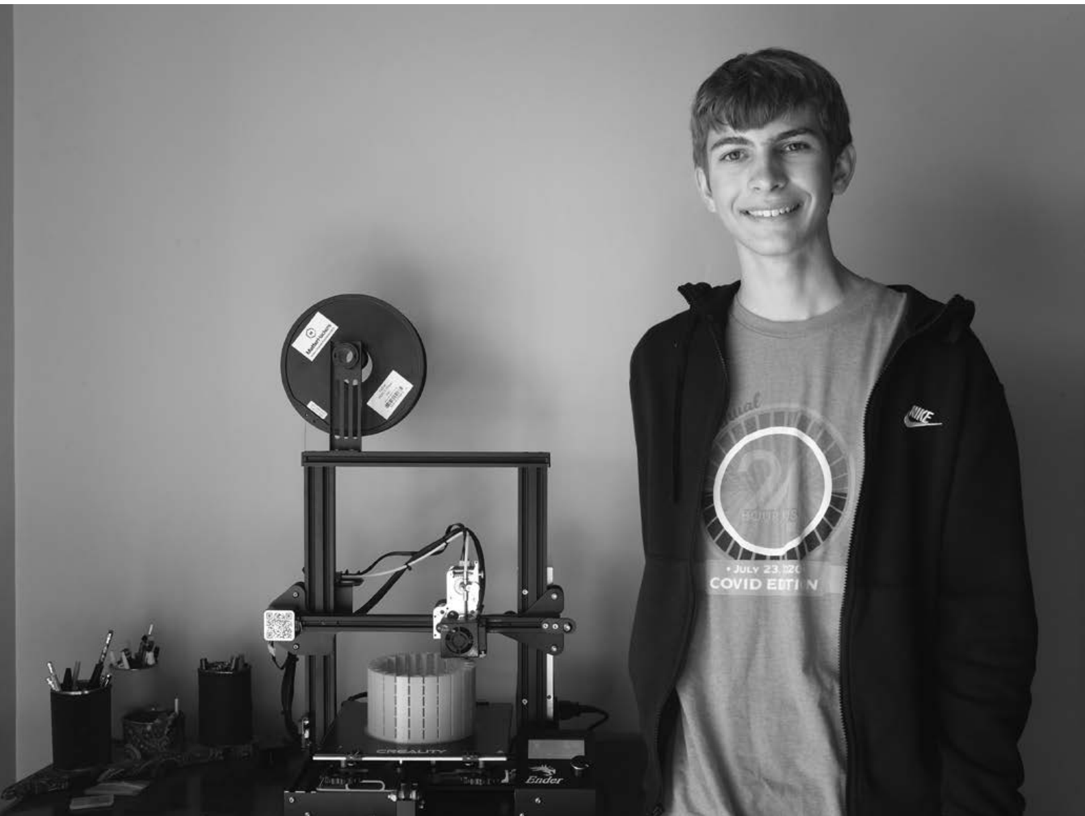
Malachi DeHaan and his 3D printer, which lays molten plastic to make a sieve for silphium seeds. Their unusual shape doesn't work with conventional seed cleaners.
