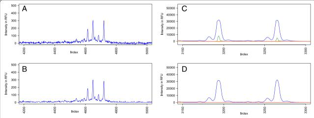
Fig. 1 Effect of Fourier transformation on smoothing and pull up correction during fragment data analysis using *Fragman*. **a** Raw data extracted from the FSA file and (**b**) data treated after Fourier transformation. Raw peak prior to (**c**) and after (**d**) pull up correction to decrease noise between channels
